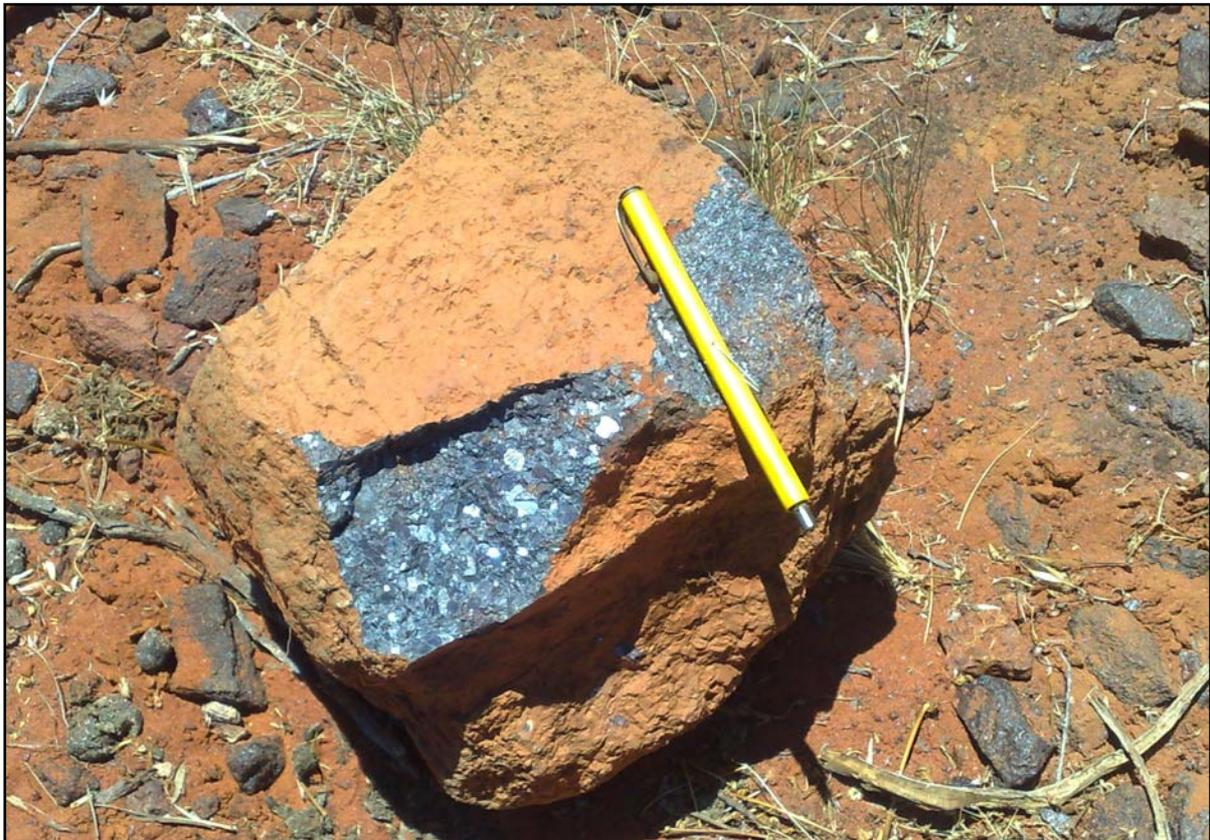
**Figure 3 – Specular hematite sample collected near North Fingerpost Hill.**
