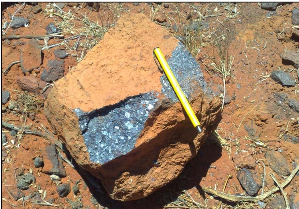
**Figure 6 – Specular hematite float sample collected near North Fingerpost Hill.**
