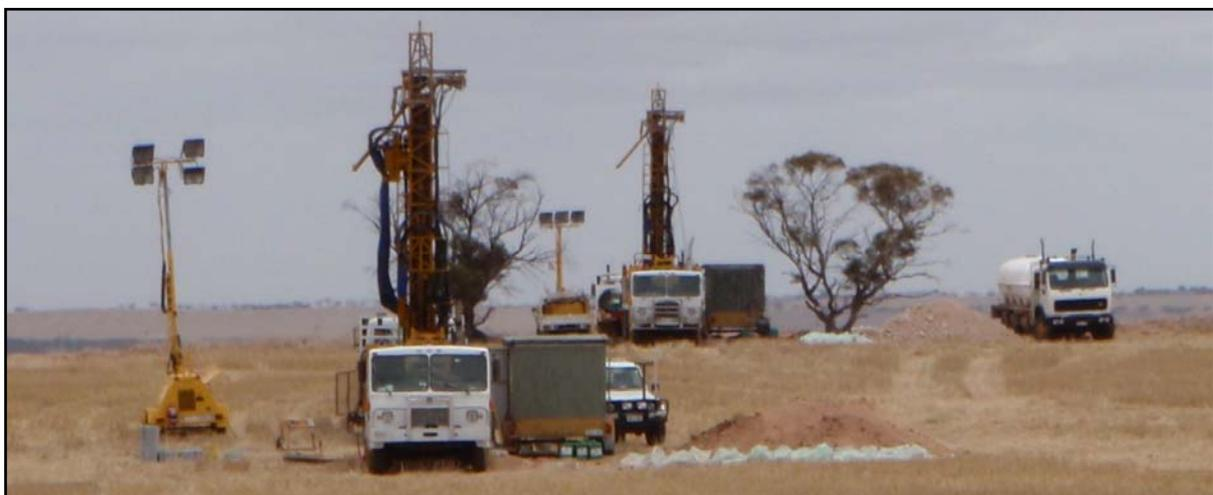
Figure 1 – Diamond drilling at Boo-Loo West, Central Eyre Iron Project.
