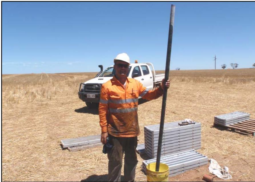
**Figure 2 – Alan Rose, Coughlan Drilling, holding magnetite gneiss diamond core with typical high competency and recovery.**
