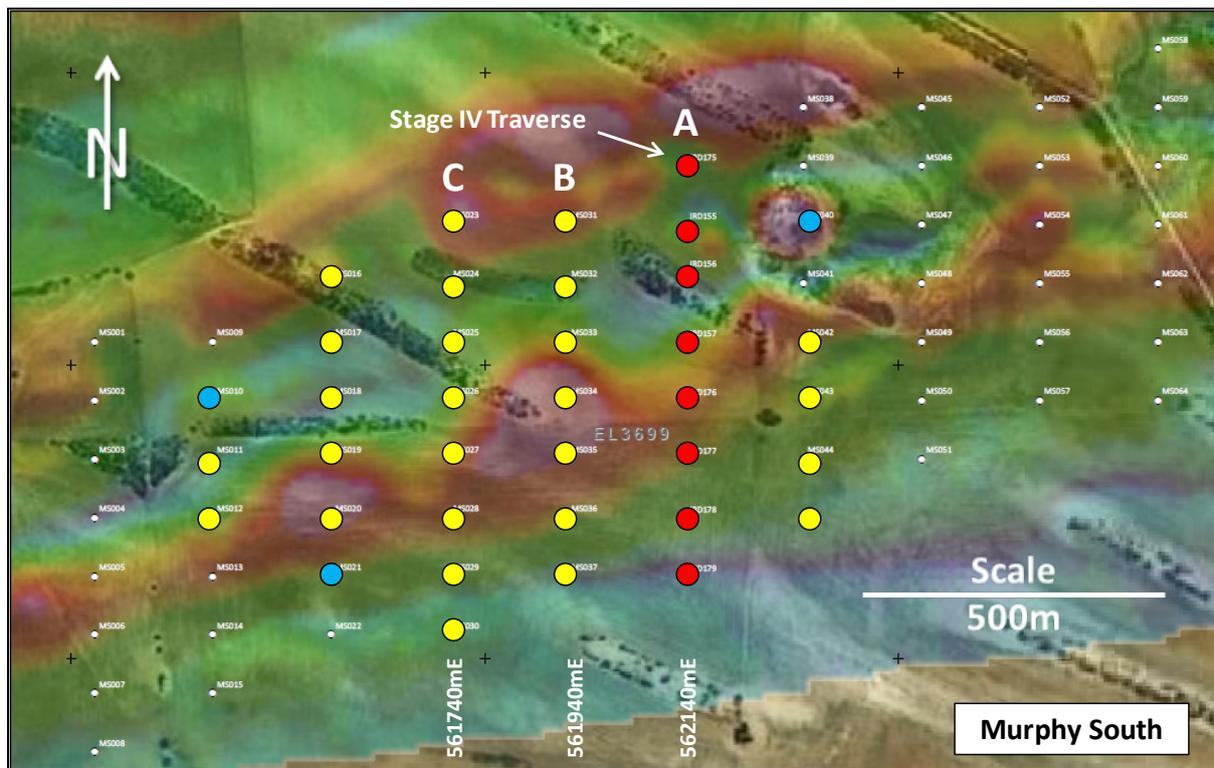
**Figure 1 – Plan view of Central Eyre Iron Project (CEIP) Murphy South Stage V Resource drilling progress. Stage IV holes shown in red, holes complete under current programme in yellow and diamond holes in progress in blue. Traverses marked A, B and C are presented overleaf in cross-section.**
