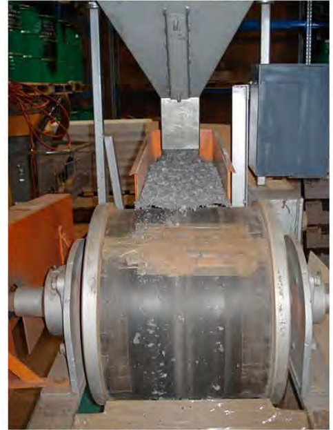
Dry magnetic separation test work
