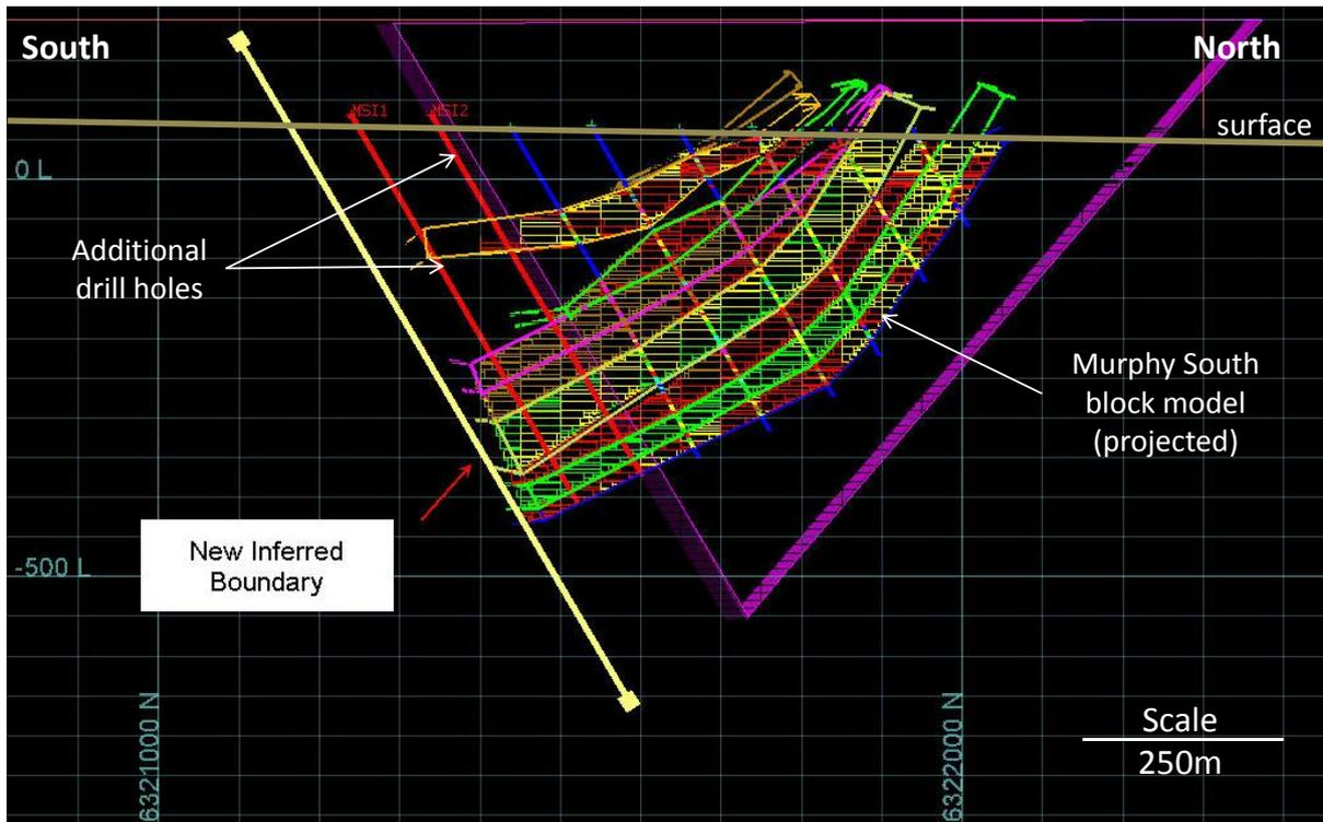
**Figure 4** Cross-section of Murphy South (562740mE) looking west showing the position of two additional drill holes (red) to allow for the extension of the resource block model down dip.
