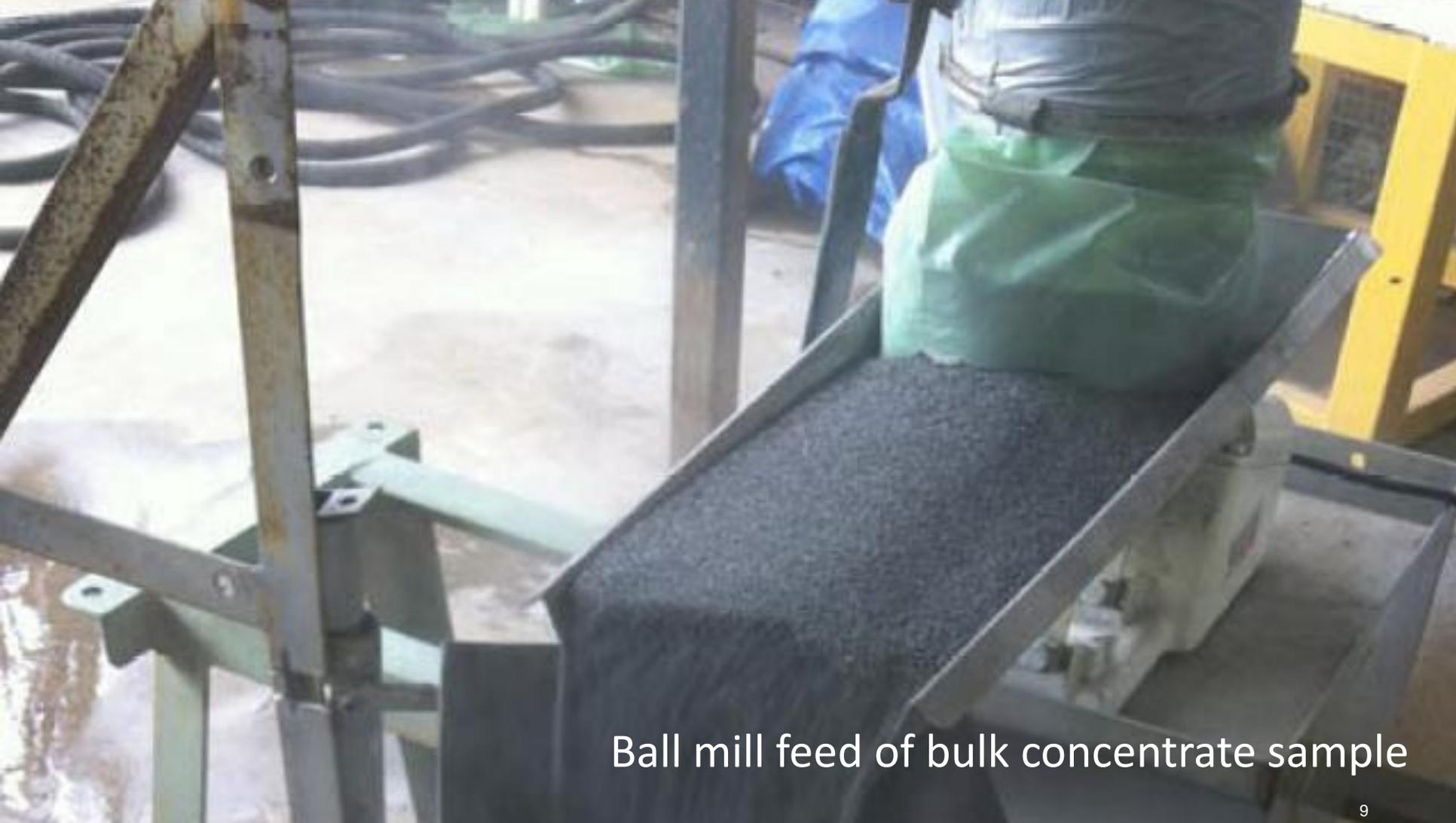
Ball mill feed of bulk concentrate sample
