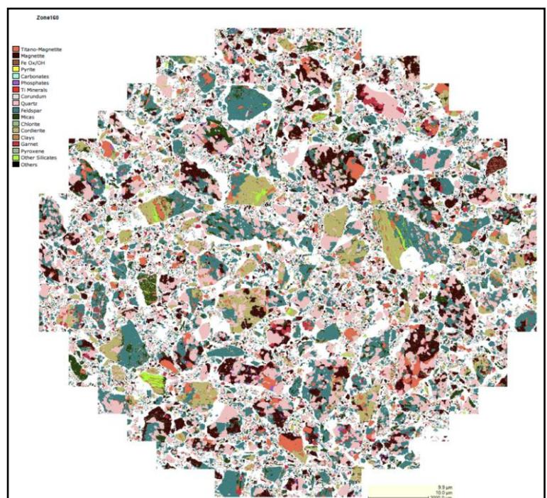
Figure 5. QEMSCAN image indicating mineral composition from the CEIP magnetite gneiss.
