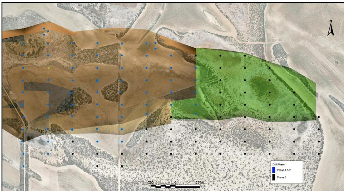
Figure 8. Rob Roy prospect showing actual (orange) and projected (green) orebody solids model
