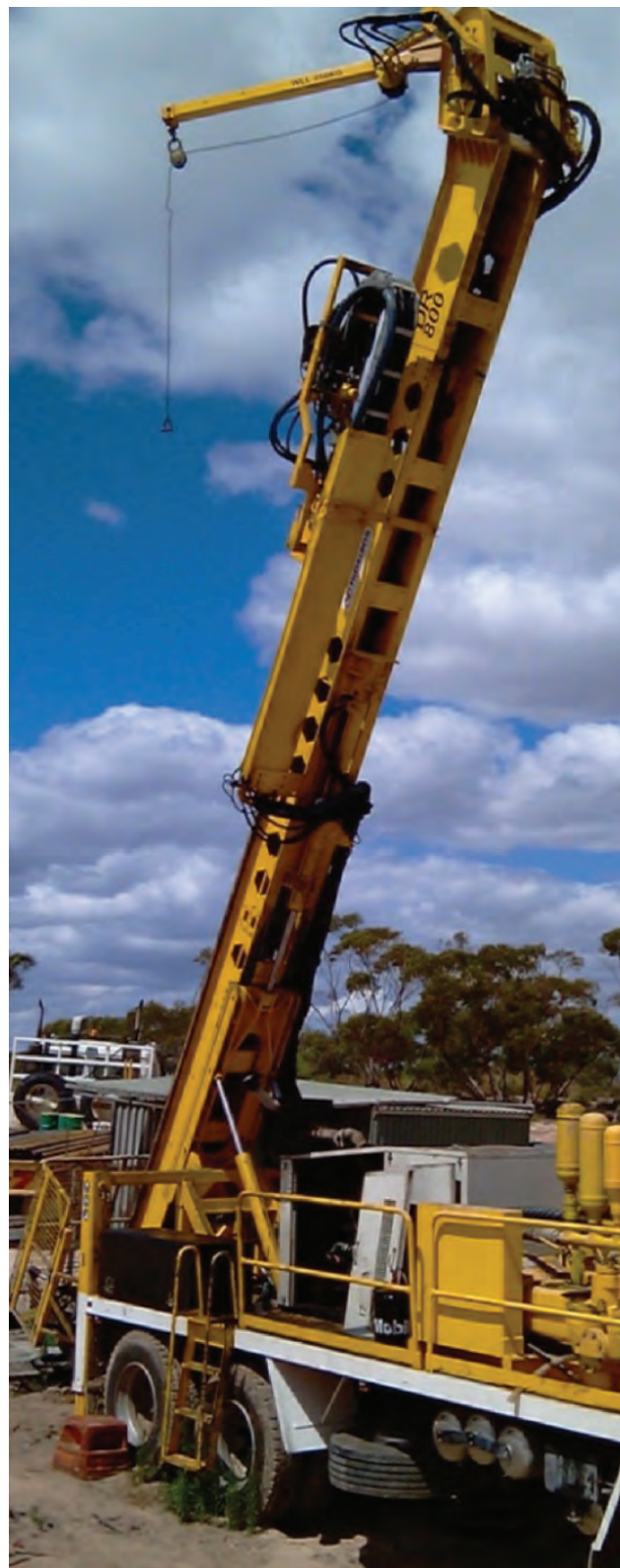
Figure 14. Diamond drilling at the Hambidge prospect
