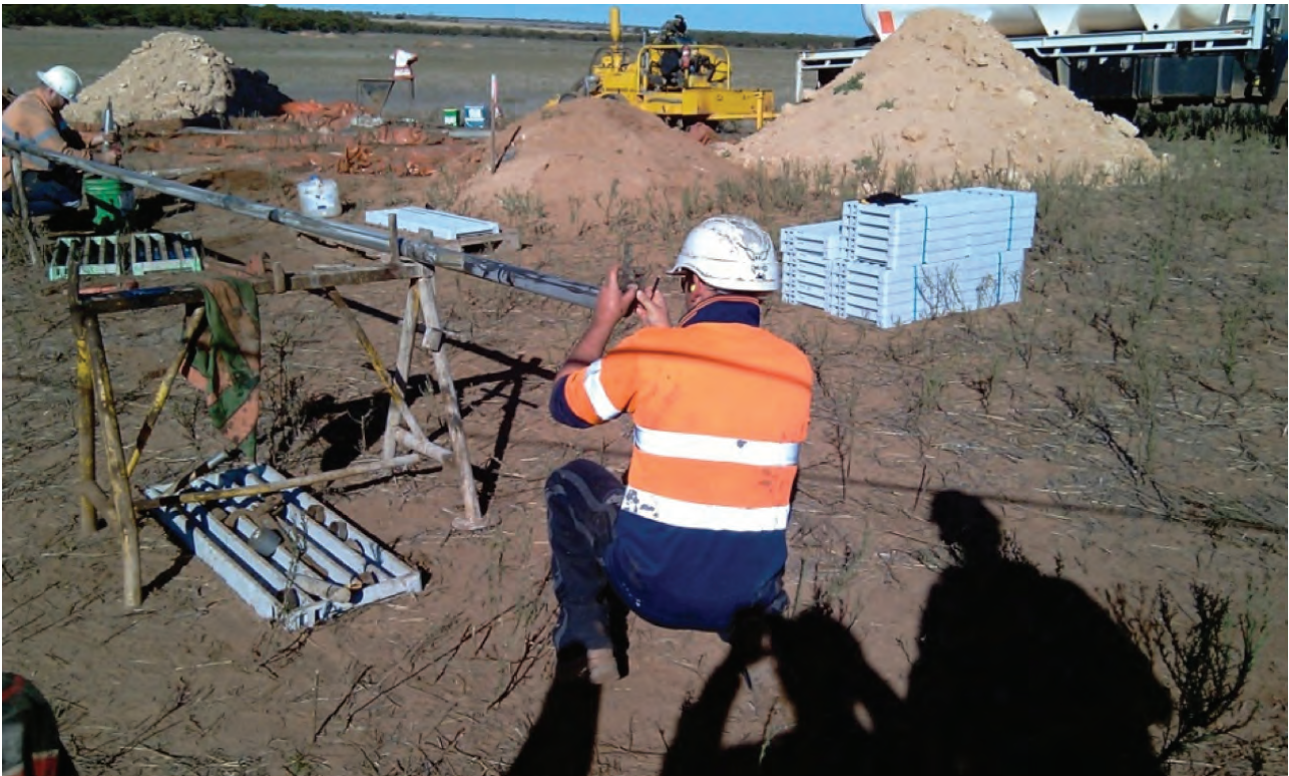
Figure 9. Orientation of drill core at Stage VII – Rob Roy
