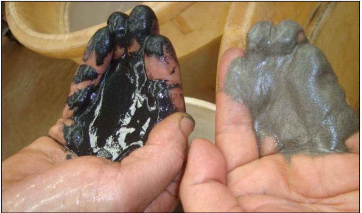
Figure 2 Wet LIMS -106µm product (concentrate) and tailings (waste)
