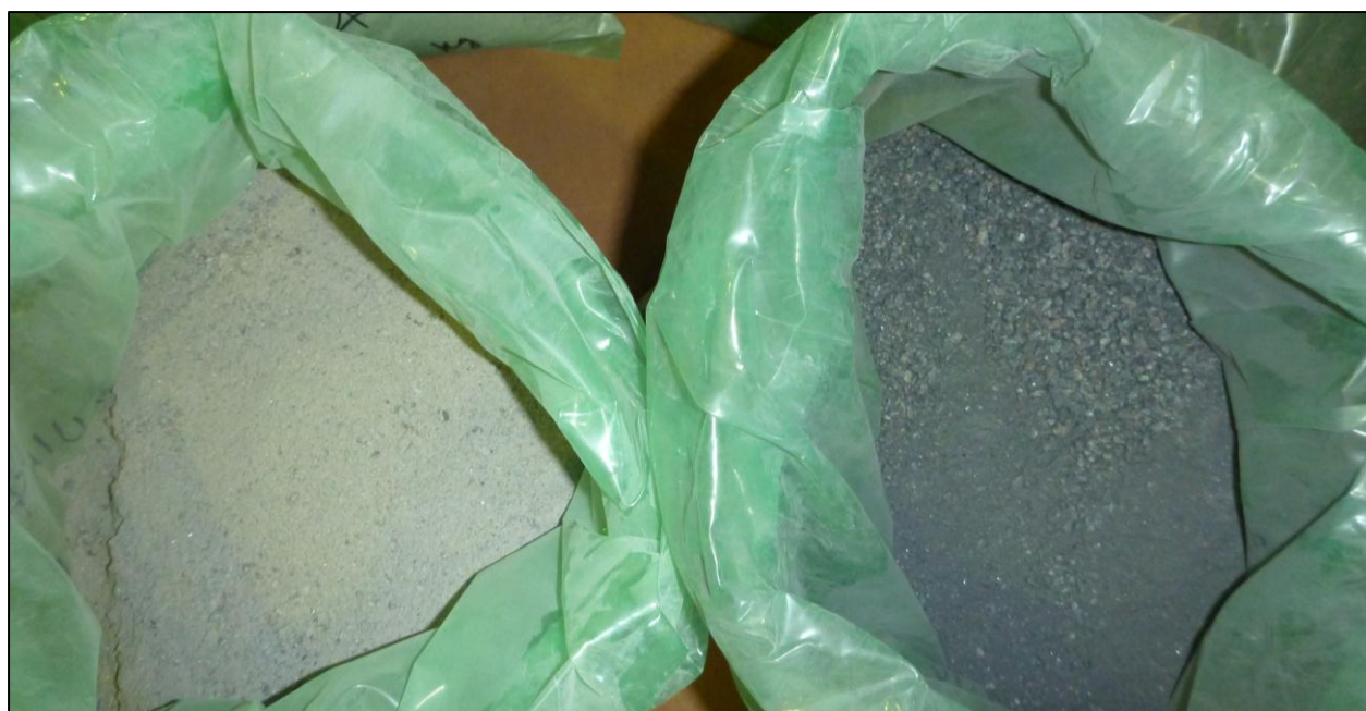
Figure 5 CEIP dried tails and coarse iron concentrate recovered during pilot RLIMS metallurgical test work
