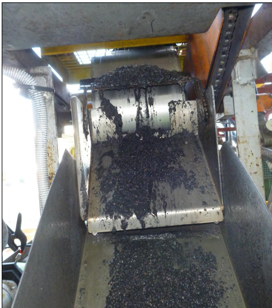
Figure 4 Coarse CEIP iron concentrate recovered during pilot RLIMS metallurgical test work.
