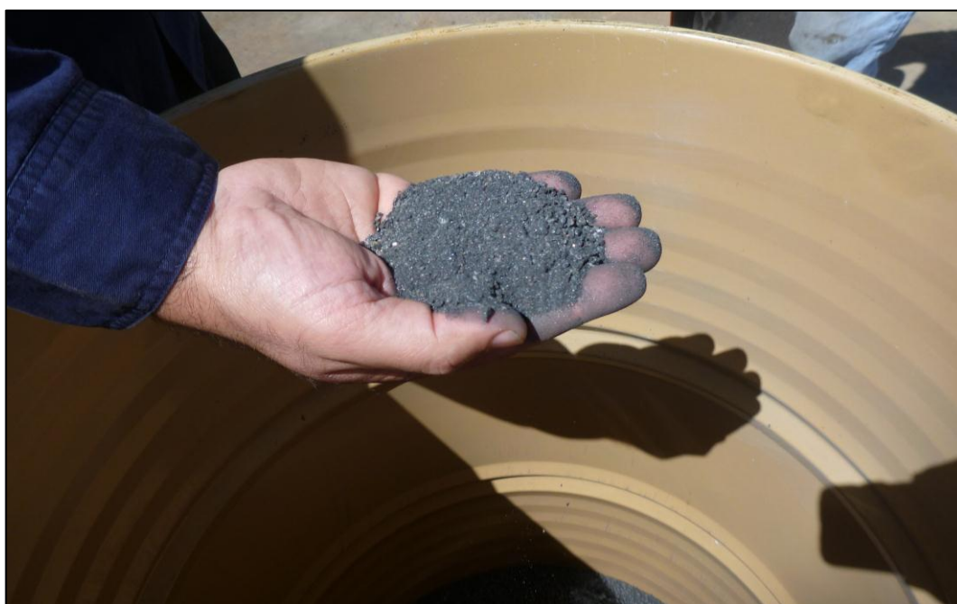
Figure 1 Coarse CEIP iron concentrate recovered from pilot RLIMS test work
