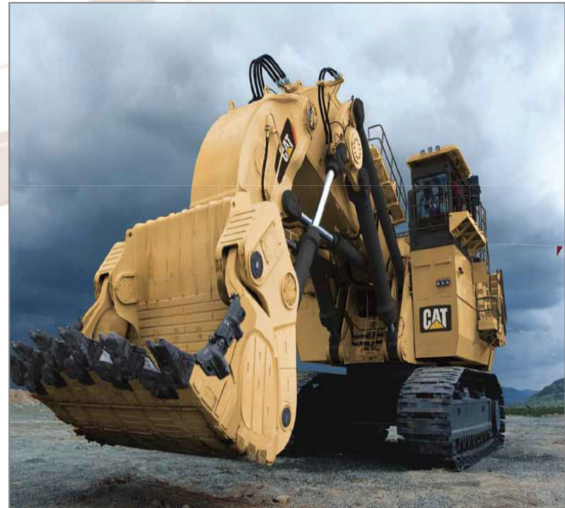
Typical excavator Cat 6090, 980 tonne machine
