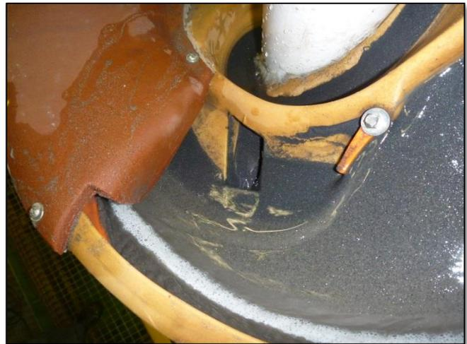
**Figure 3 – Full scale rougher spiral test showing darker magnetite concentrate being split from the particle stream on the spiral.**
