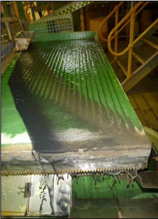
**Figure 2 – Shaking table test showing characteristic clean separation between magnetite (dark stream of particles on the left) and gangue (sandy coloured stream of particles on the right).**
