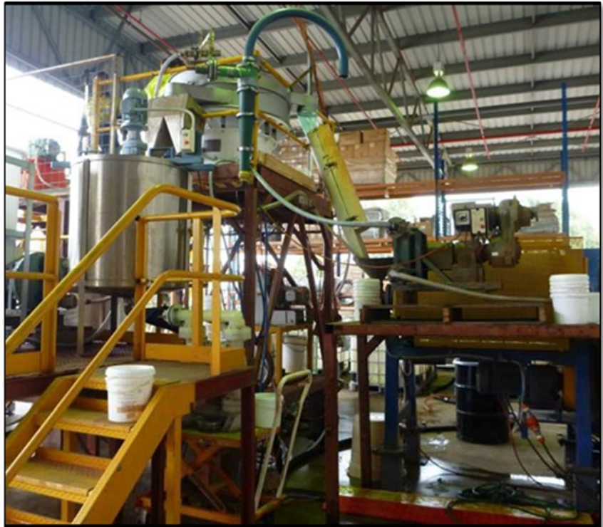
Figure 14 Pilot milling circuit in operation at Amdel. The mill is located within the yellow guarding in centre right of the picture.
