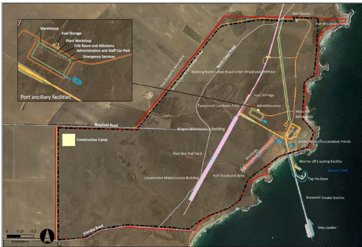
Figure 10 Current port layout at Cape Hardy including tug harbour and module offloading facilities (MOF).
