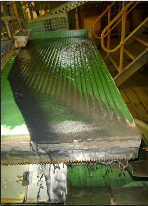
Figure 6 Shaking table test showing characteristic clean separation between the magnetite-hematite concentrate (dark stream on the left) and gangue (sandy coloured stream on the right).
