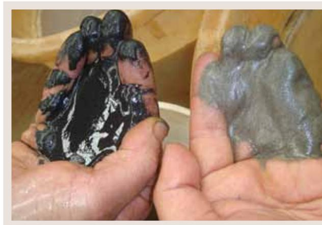
Figure 13: Final concentrate (left) and cleaner magnetic separation tails (right)
