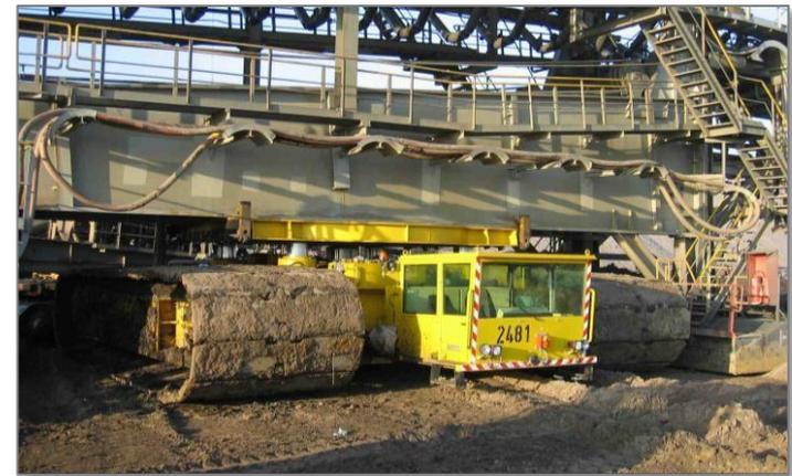
*At right: Semi-mobile gyrotory crusher station in Sweden, similar capacity required at CEIP. Below, transport crawler undertakes conveyor system reconfiguration*
