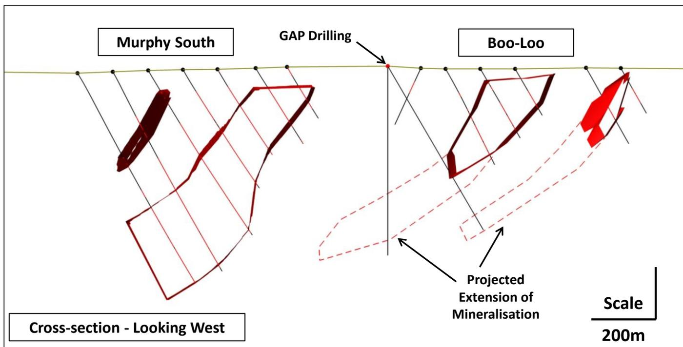
**Figure 2-** Section 559740E looking west showing Murphy South and Boo-Loo mineralisation. The proposed holes are shown with the expected GAP target delineated by the dashed red lines.
