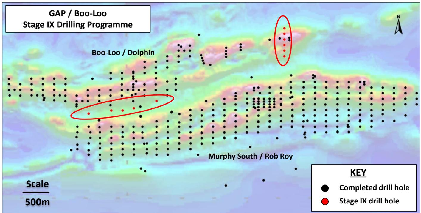
Figure 1 Plan view of CEIP Boo-Loo - Dolphin, Murphy South and Rob Roy drill collars superimposed on aeromagnetic image. Stage IX collars in red.
