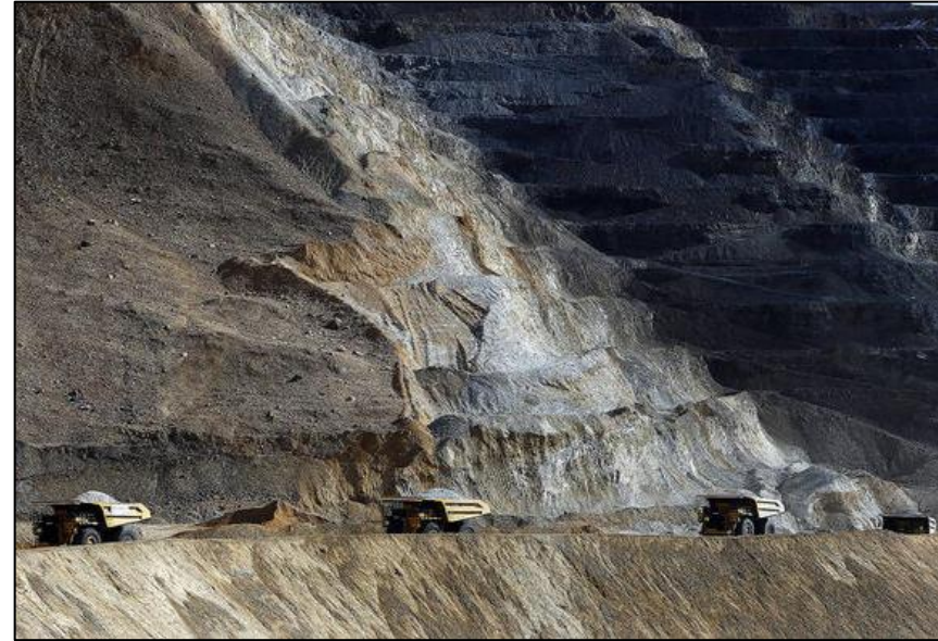
Conventional truck and shovel open pit mining operation
