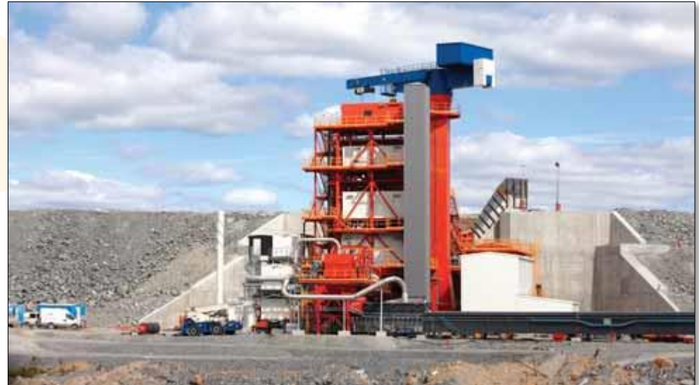
Boliden's Aitik Copper Mine in Sweden uses semi-mobile crushers
