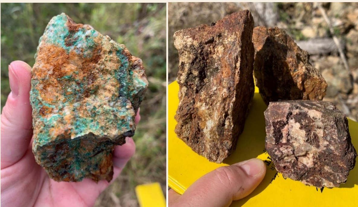
Figure 1. Sample MRRK071, 3.49g/t Au, 2.8% Cu & 195g/t Ag (left). Sample MRRK072, 6.06g/t Au, 585g/t Ag, 1.5% Cu, and 3.58% Sb (right)
