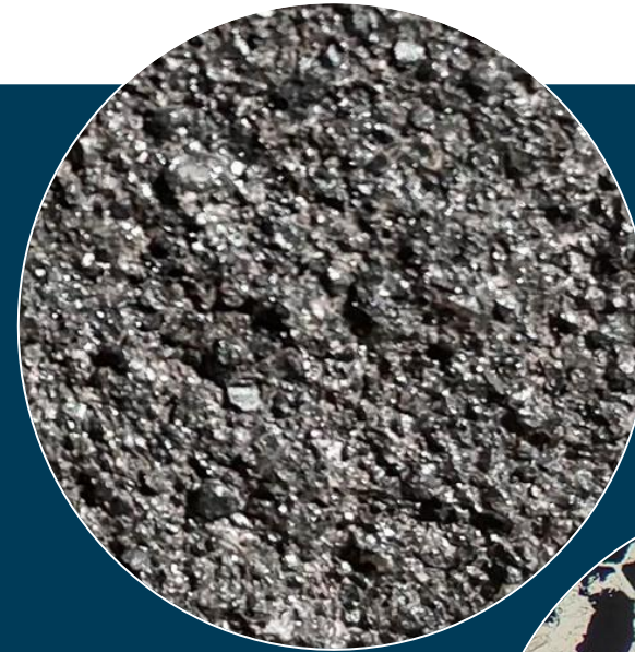
Sub-euhedral magnetite ranging in size from 0.1mm – 5mm
