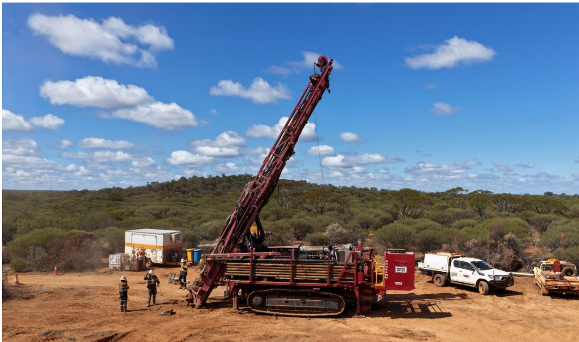
Figure 6: RC drilling at Killi Resources' Lodestone Iron Ore Project.
