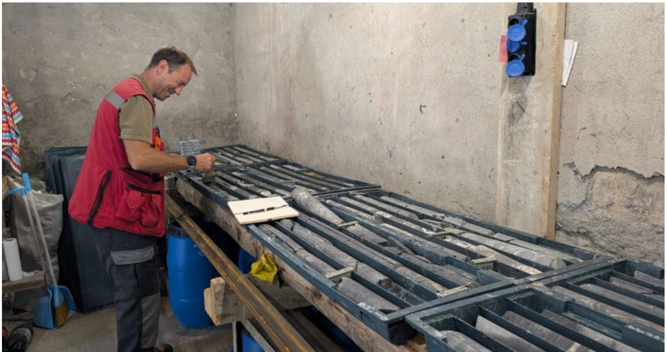
Figure 7 Photo of resource consultant geologist inspecting the core from 2025 and 2026 drill programs
