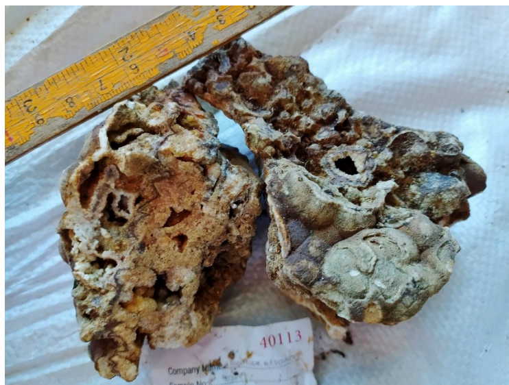
Figure 4: Rock float (SN# 40113) from Kimono Central displaying comb, crustiform, colloform, lattice bladed and botryoidal quartz textures typical of the boiling zone of an epithermal system
