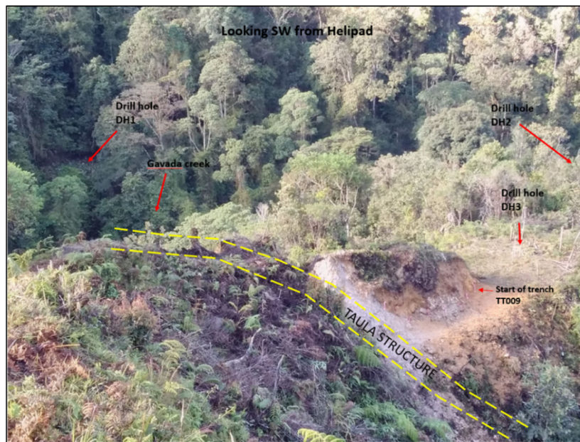
Figure 17: Taula Structure at Trench TT009 with 8m @ 2.83g/t Au including 1m @ 11.15g/t Au.
