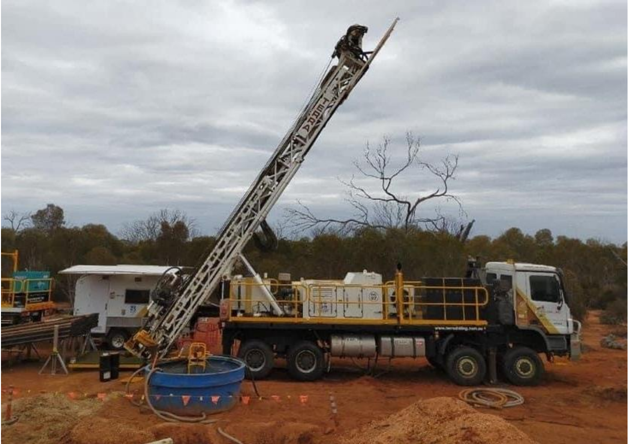
Figure 2: Terra Drilling diamond drilling rig on site at Lady Grey Project Mt Holland
