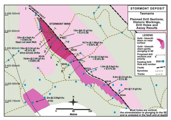
Diamond saw sampling along the strike of the open pit wall previously returned 32m grading 4.8 g/t gold + 0.56% bismuth, and sampling in a cross cut returned 10m grading 5.34 g/t gold +0.31% bismuth and also showed the adit was terminated in greater than 1 ounce/tonne gold. Frontier undertook vertical channel sampling in the open cut plus horizontal channel sampling in the adit to confirm these grades.
