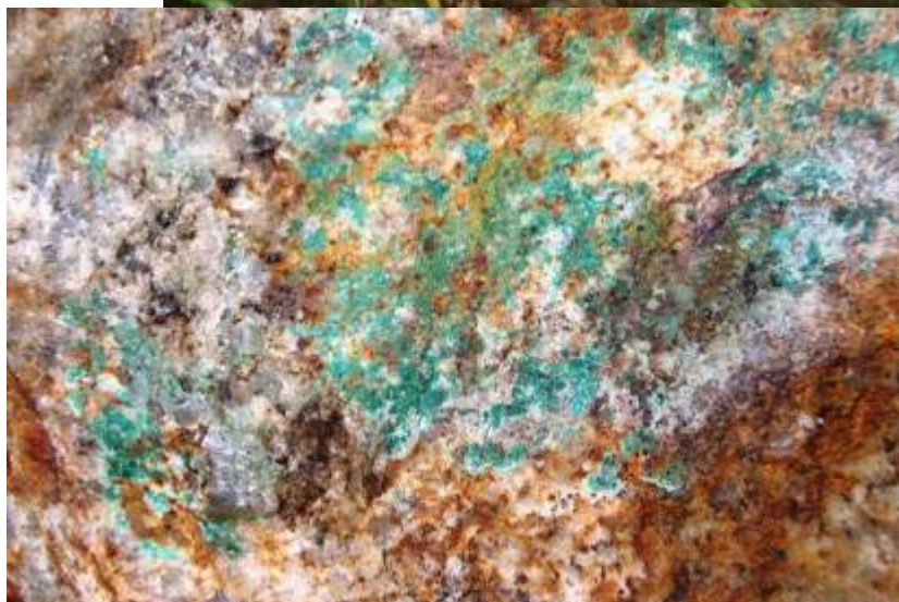
Figure 16. Secondary copper mineralisation on the fracture face of a porphyritic rock from Andewa at approx. real (100%) scale.
