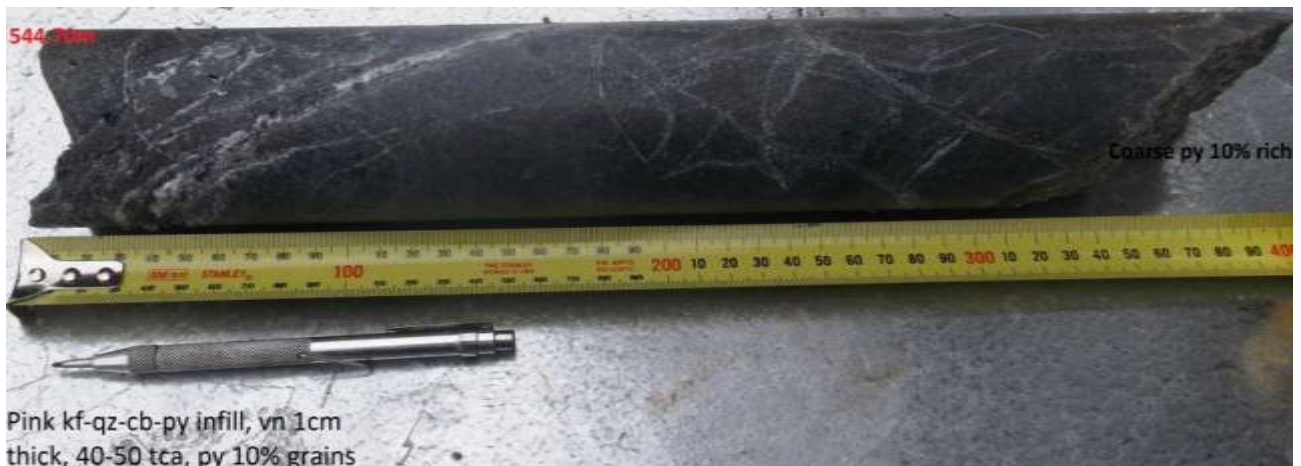
Photo 3: Vein infill with coarse pyrite grains, up to 10% angled between 40-50° to core axis.
