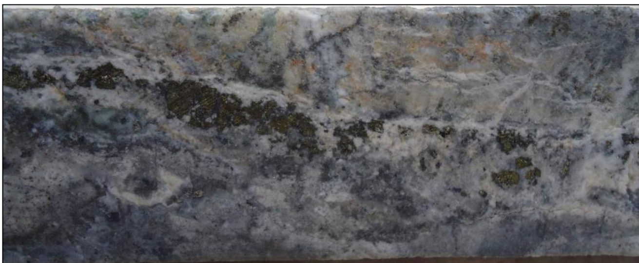
Chalcopyrite-molybdenite blebs on vein in brecciated clasts within the shear zone.
