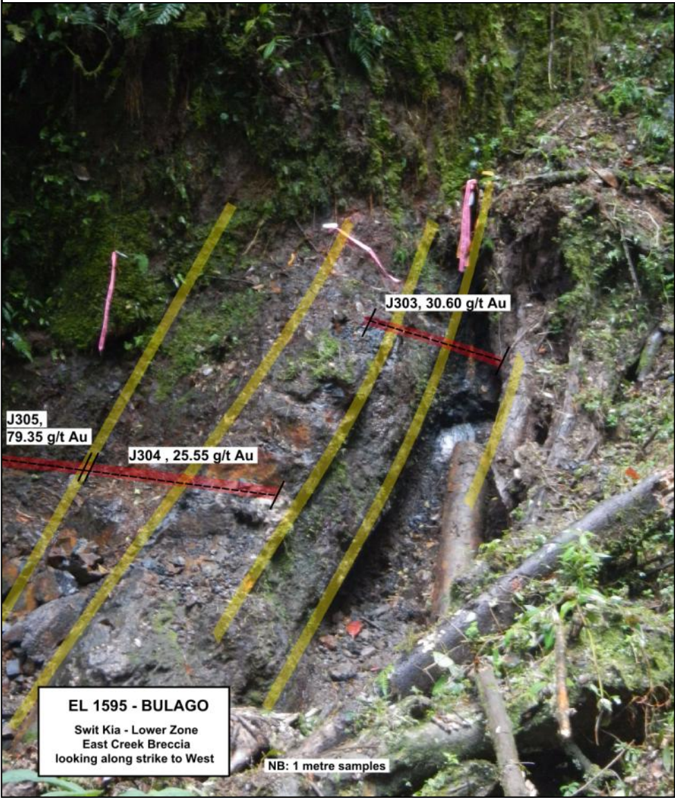
Photo 11. The East Creek breccia looking along strike to the WNW showing the moderate-high angle plunge or dip (?) to the SW, with 1.0m grading 79.35 g/t gold, within 3m grading 45.17 g/t gold (J303, J304 and J305). Unfortunately, the photo didn't capture the highest grade zone very well.
