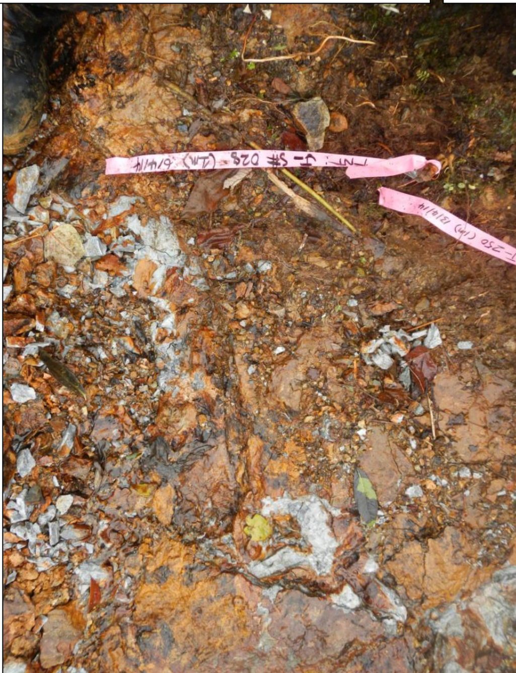
Photo 7. Sample J-028 from Trench 1 with 222.0 g/t gold, crossing near Trench 7 sample J-250, with 155.5 g/t gold.
