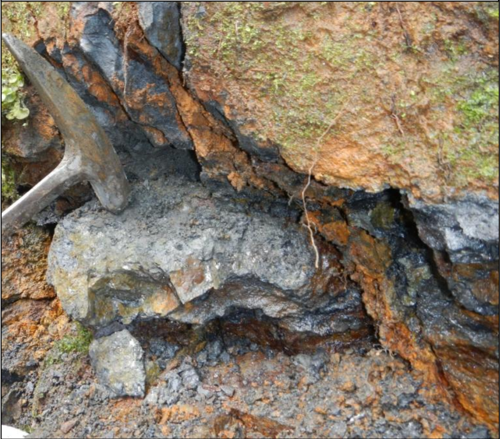
Photo 13. The highly sulphidic breccia and quartz veining with 0.40m grading 297 g/t gold outcrop (J 416).
