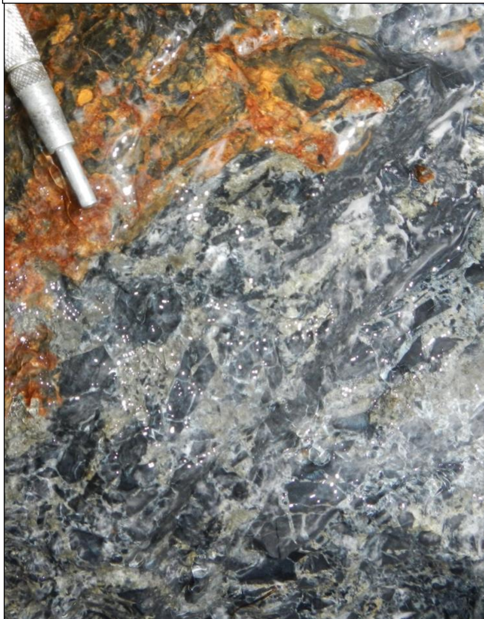
Photo 10. Grab Sample G002 - a magnificent hydrothermal breccia in siltstone from East Creek (with only 7.98 g/t gold + 43.2 g/t silver), that documents the western strike extension of the Upper Zone. More intensely mineralised intrusive is likely to be very nearby subsurface based on the mineralisation model.
