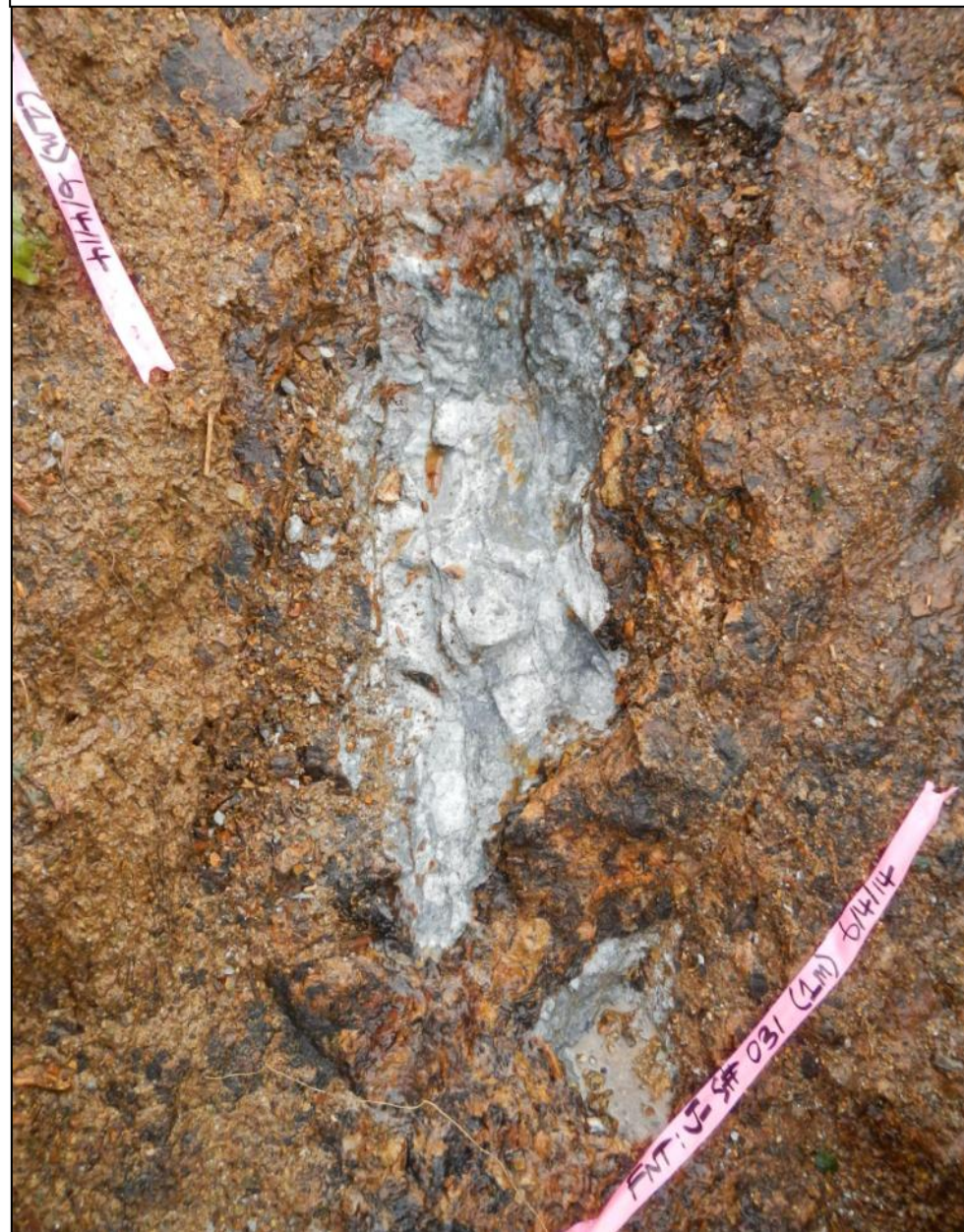
Photo 4. Sample J-031 from Trench 1, with 163.0 g/t gold in gravimetric analysis, but 38.0 g/t gold in 50 gram fire assay. This was the only significant 'anomaly' or difference between the 2 types of analyses.
