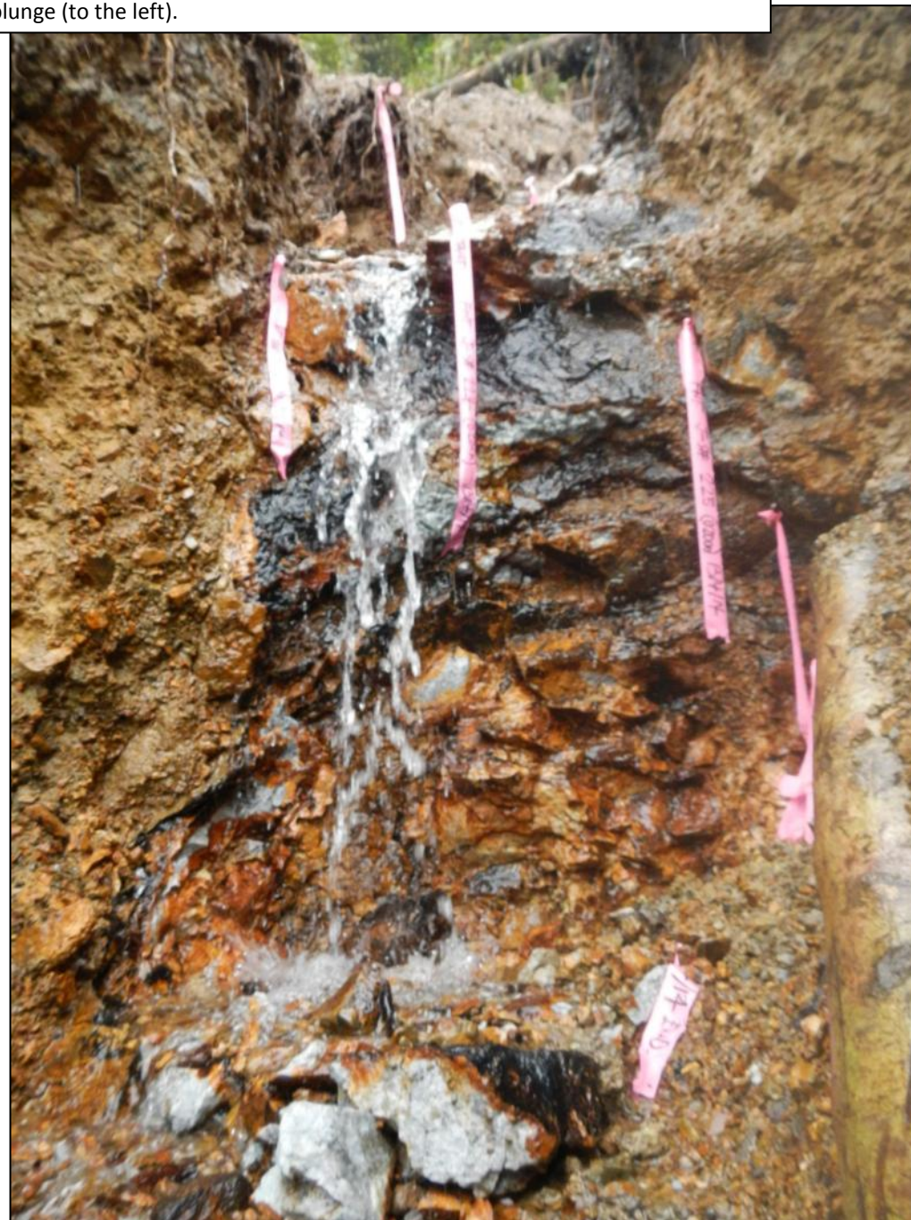
Photo 8. Pit 1 showing samples J-224-228 (18.70 to 0.10 g/t gold) and an apparent shallow SW plunge (to the left).
