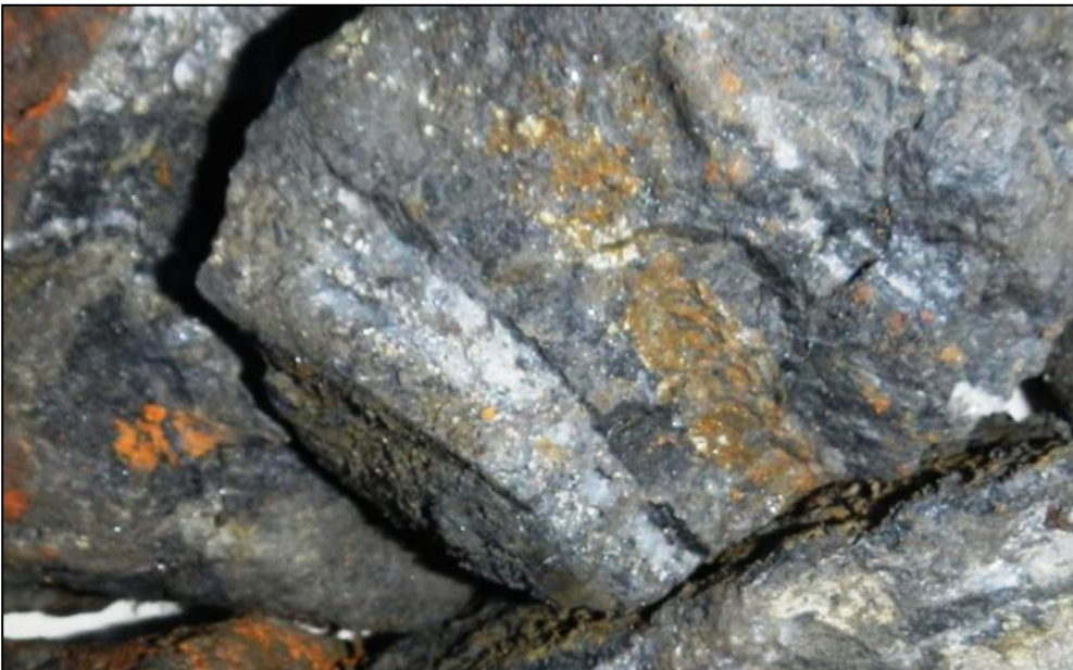
Photo 15. Strongly sulphidic (pyrite, arsenopyrite, sphalerite and galena) and silicified conformable gold mineralisation from the Lower Zone at J400, with 0.3m grading 197 g/t gold
