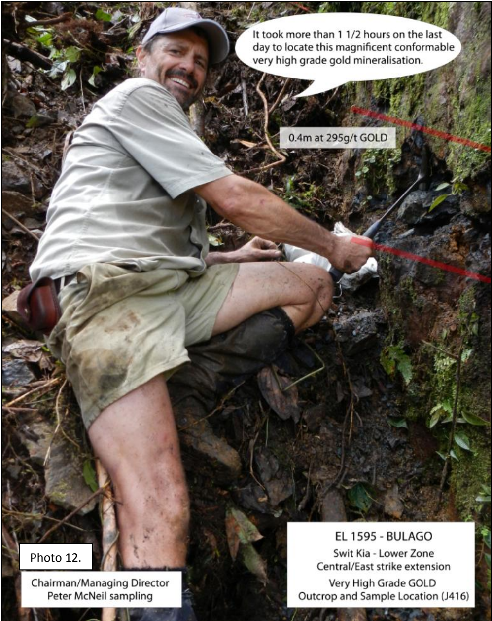
Photo 13. The highly sulphidic breccia and quartz veining with 0.40m grading 297 g/t gold outcrop (J 416).
