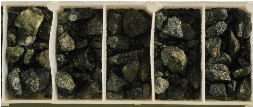
Figure 2: Magnetic Gabbro hosted mineralisation in RC chips, TBRC062 165-170m (Turnberry Central). The pictured interval represents 5m @ 14.9g/t Au within a wider 41m @ 4.8g/t Au interval. Alteration is Chlorite-Pyrite(3%)-Epidote-Carbonate.
