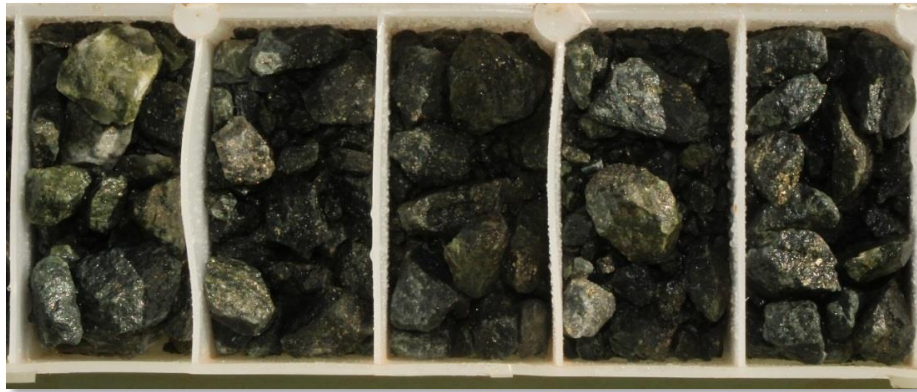
Figure 3: Magnetic Gabbro hosted mineralisation in RC chips, TBRC062 165-170m (Turnberry Central). The pictured interval represents 5m @ 14.9g/t Au within a wider 41m @ 4.8g/t Au interval. Alteration is Chlorite-Pyrite(3%)-Epidote-Carbonate.
