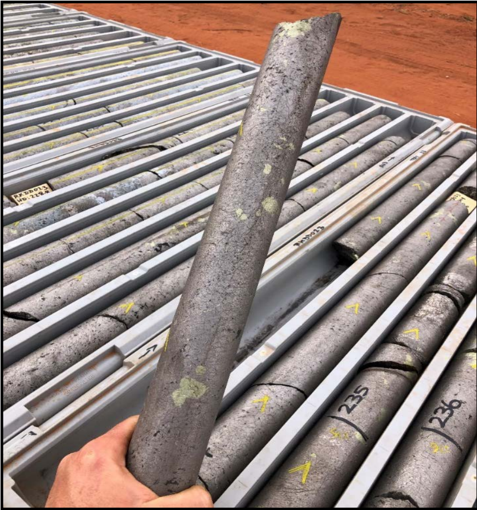
Massive Ni-Cu Sulphide from RKDD023 from 233m, NQ2
