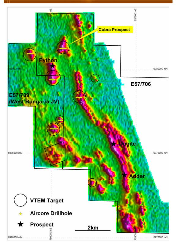
Figure 2: Bungarra VTEM Image (Channel 34) with Aircore Drillholes
