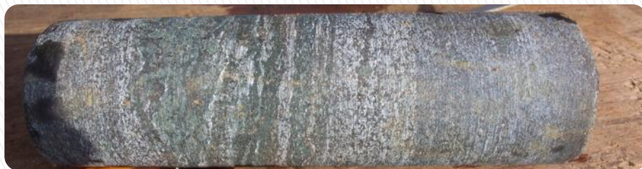
Magnetite Gneiss Core – Hole NESD011 (sample MET1)
