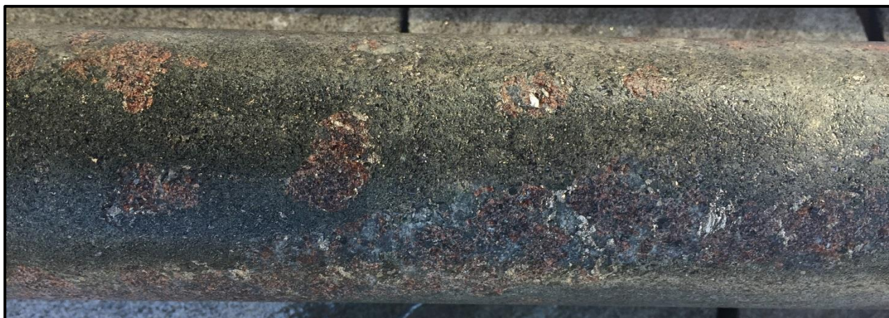
Photo 3: Sulphide in pyroxene-garnet-feldspar lithology, 739.3m (NQ2 core)
