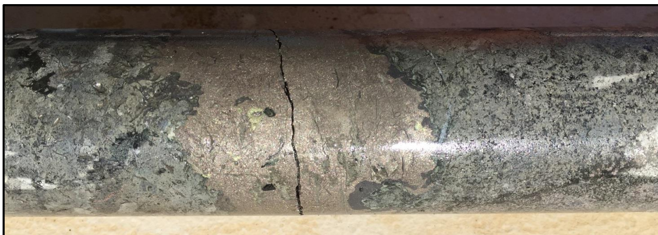
Photo 1: Massive pyrrhotite, minor chalcopryite in pyroxenite, 694.5m (NQ2 core)
