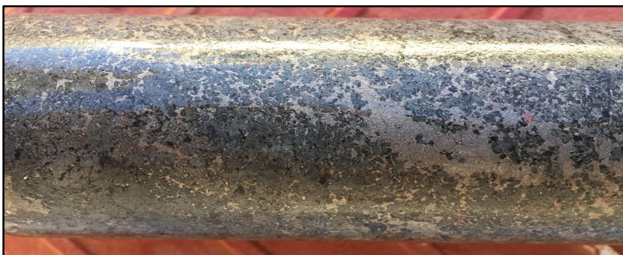
Photo 2: Matrix pyrrhotite, minor chalcopryite in pyroxenite, 693.9m (NQ2 core)
