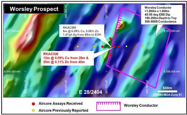
Figure 3: Worsley Aircore Drillholes and MLTEM Conductor on Aeromagnetics
