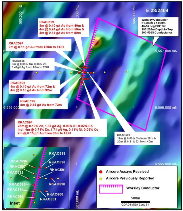
Figure 2: Worsley Aircore Drillholes and MLTEM Conductor on Aeromagnetics
