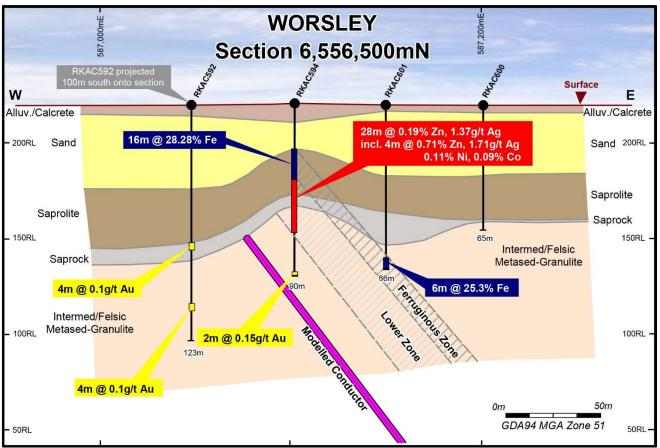
Figure 3: Drill Section 6,556,500N Showing Anomalous Geochemical Zones Relative to Position of Modelled MLTEM Conductor
