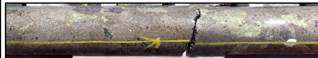
Massive pyrrhotite-chalcopyrite-pentlandite sulphide in drillhole RKDD007, 119m (NQ2 core)
