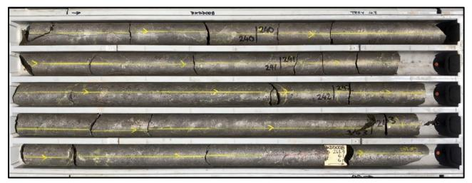
Photo: Diamond Drillhole RKDD008 – 4.5m interval (239.5-244.0m) from larger 12.8m massive nickel-copper sulphide intersection (234.9-247.7m) (NQ2 core)
