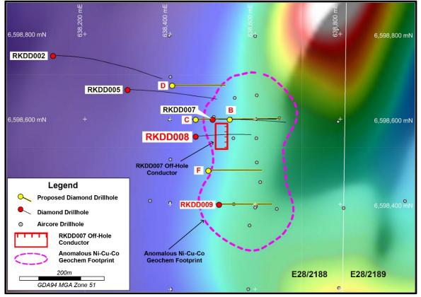
Figure 1: RKDD008 and Proposed Diamond Drillhole Locations on Aeromagnetics
