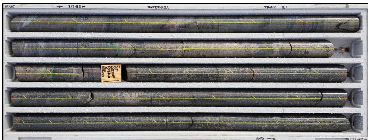
Semi-massive and net-textured Ni-Cu sulphide mineralisation, RKDD021 219.1m-222.52m, NQ2
