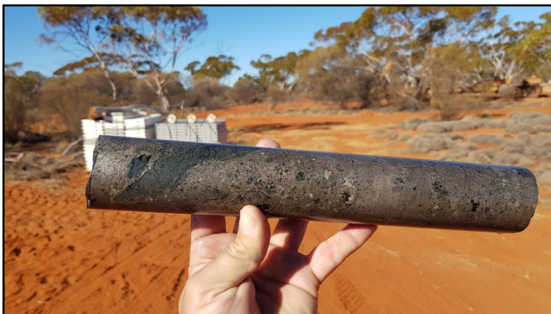
Semi-massive Ni-Cu Sulphide mineralisation from RKDD021 from 219.5m, NQ2
