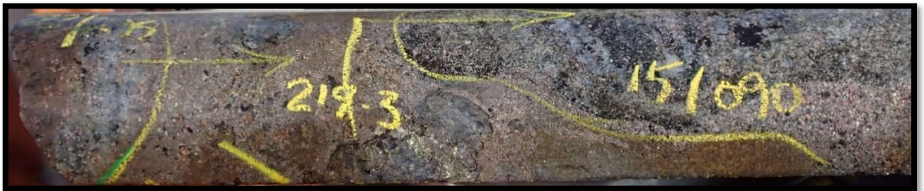
Melt Migration Texture of Massive Ni-Cu Sulphide from RKDD023 from 219m, NQ2
