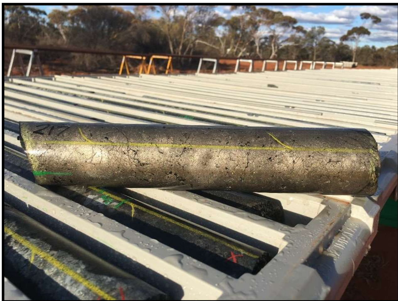
RKDD025 Massive Ni-Cu Sulphide from 217m, NQ2
