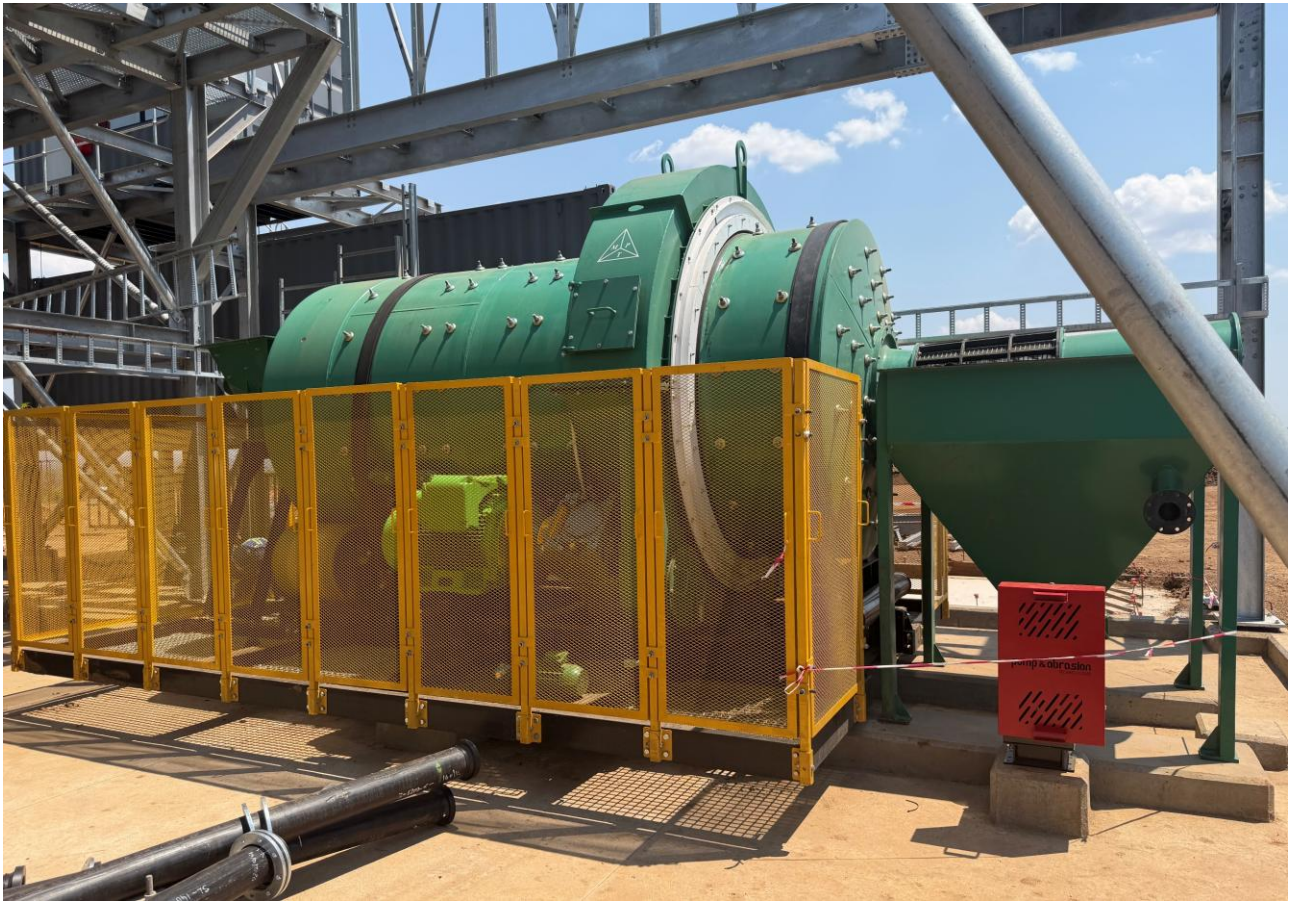
Picture 7. Regrind Mill installed at the process plant at Kangankunde
