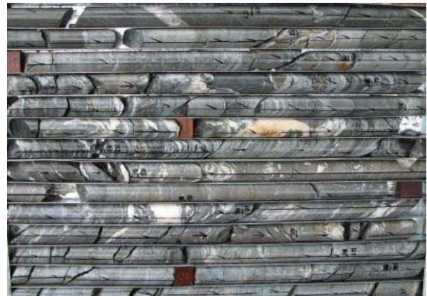
Hole LTD0023 from 162.5 to 168.5, 6 metres 8.8% zinc, 2.3% lead, 0.3% copper, 1.2 g/t gold
