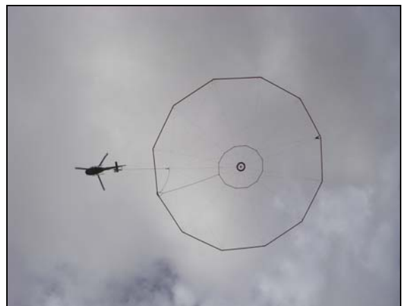
Helicopter-borne VTEM geophysical survey underway at Liontown
