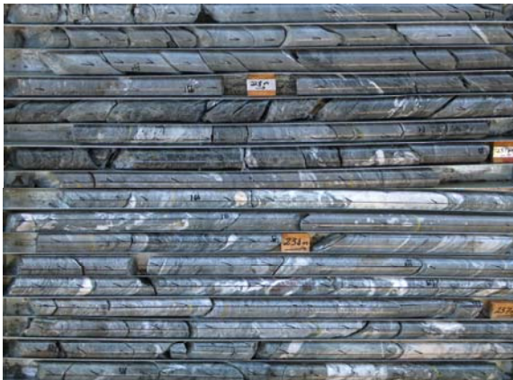
Hole LTD0009 from 230-234m, 4m @ 11.5% zinc, 3.0% lead, 0.7% copper, 34.9 g/t silver, 0.2 g/t gold
