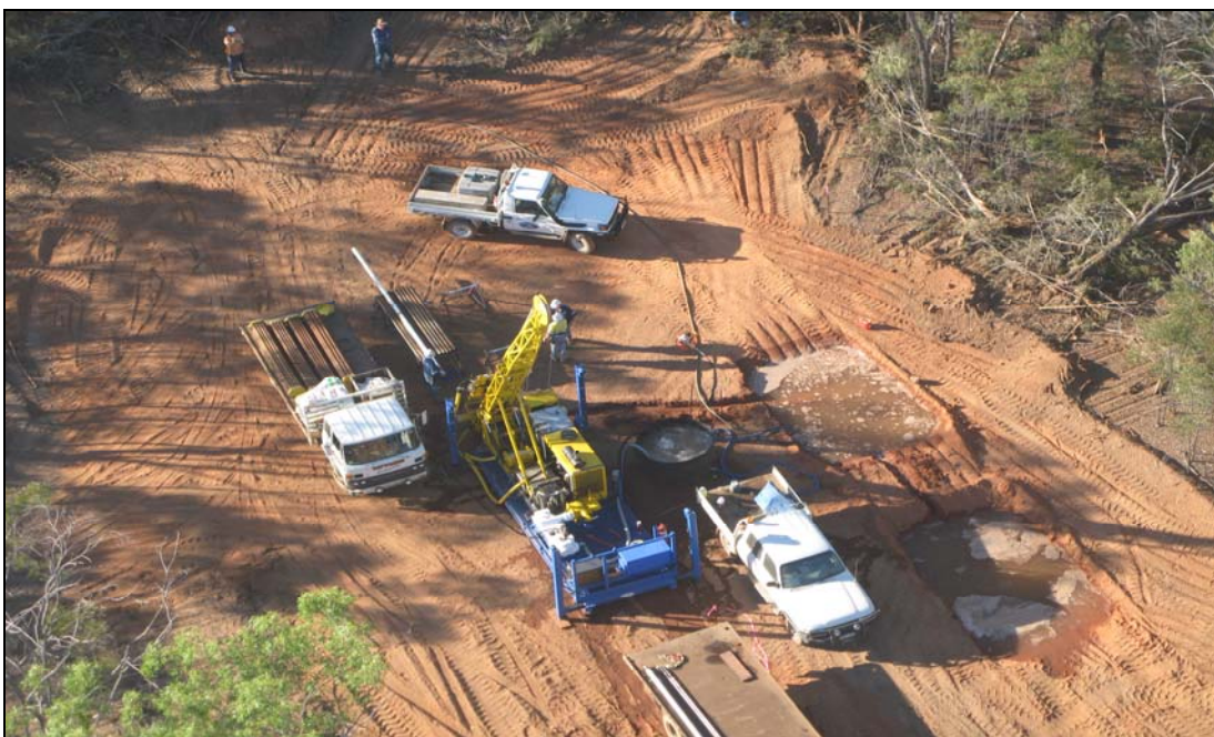
Diamond drill rig operating at Liontown
