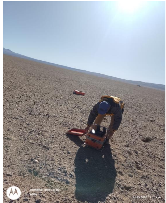
Figure 2: Placement of TEM Equipment
