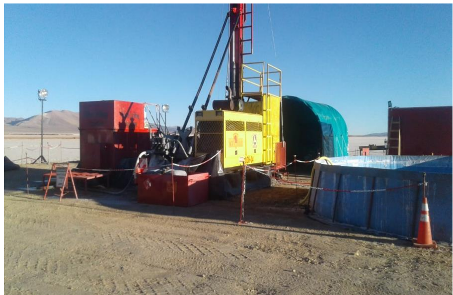
Figure 4: Typical drill rig used for drilling at a salar
