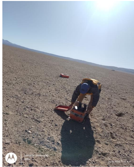
Figure 3: Placement of TEM Equipment
