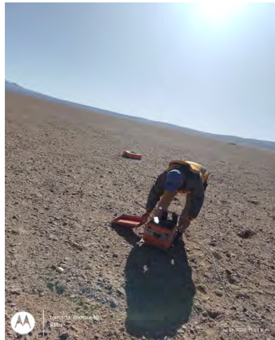
Figure 5: Placement of TEM Equipment
