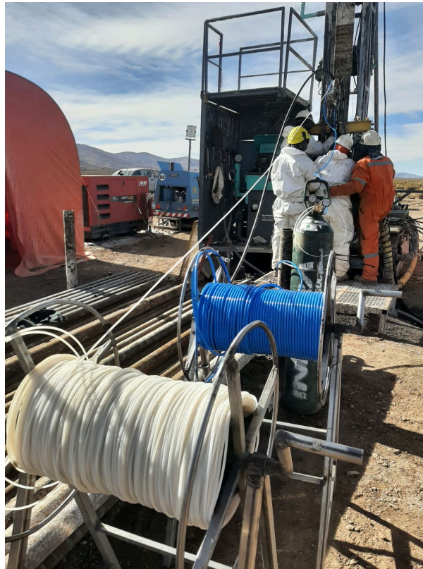
Figure 1: Packer sampling at Drillhole SOZDD001 (Mario Angel Concession)
