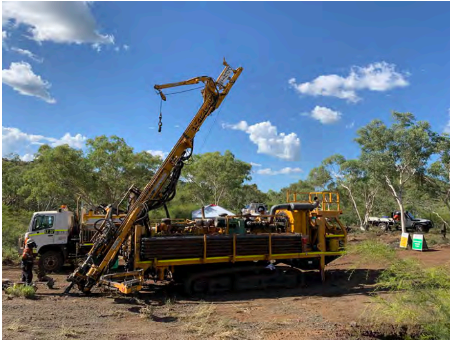
Figure 22: RC Drill Rig Mobilising on Corella Tenement
