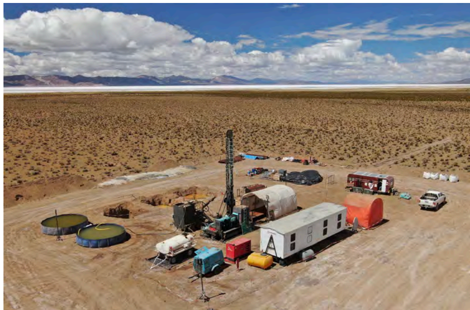
Figure 1: Diamond Drill Rig at Drill Hole 5 (SOZDD005, Chico VI Concession) on Olaroz Salar
